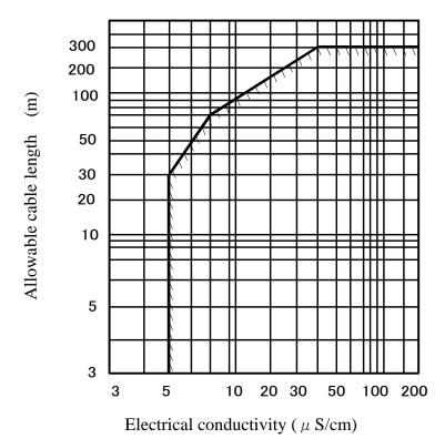
Figure 9.1 Electrical Conductivity vs. Cable Length
